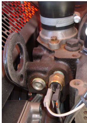
Sensor for white smoke prevention in cold starts (surcaleur)
